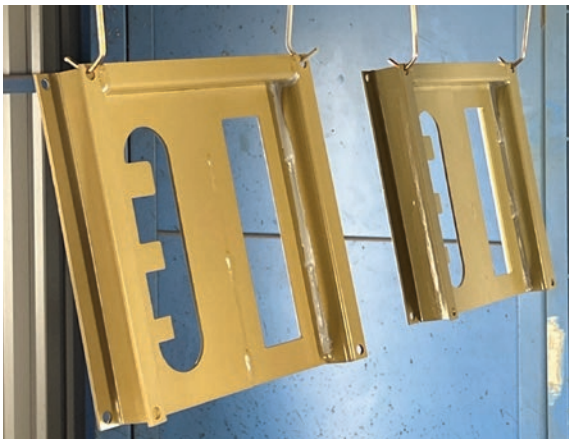
Figure 41. Test samples for steel material corrosion durability investigations.
