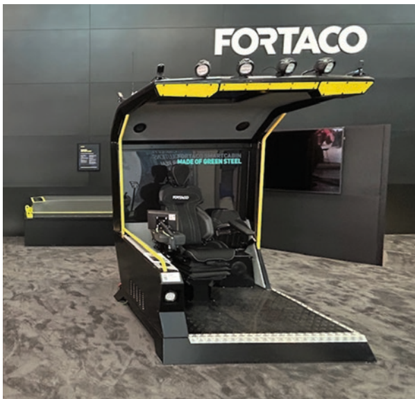
Figure 38. Exhibition cabin built with SSAB Zero™ fossil-free steel material.
